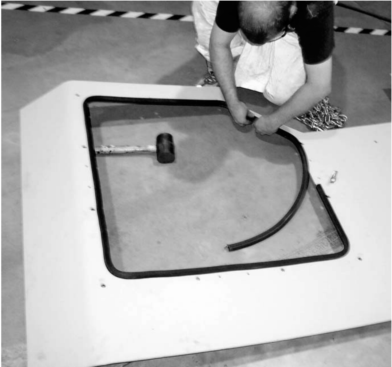
Figure 39. Installing the Escape Hatch Bulb Seal.
