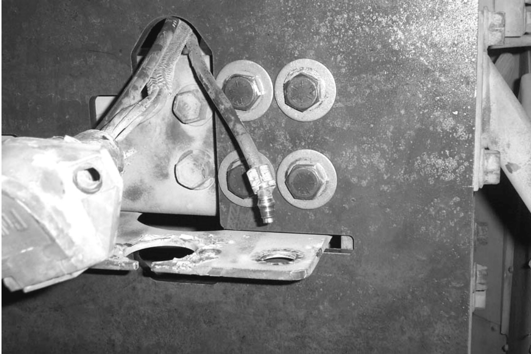
Figure 57. Routing the Glad Hand line and Electrical Connector.
